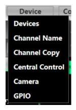
**Devices**: view or modify the software version information, device name and device IP address of the upper and lower computer of the device.
