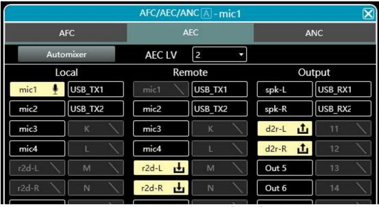
Matrix processor supports to control a certain degrees of echo from local room to remote room, which usually happened in remote video conference via network software Skype, Zoom, or via remote conference system controller(terminal). This function is mainly used for voice process.
