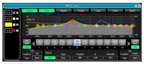
Phase curve: display the phase curve of the current channel.
