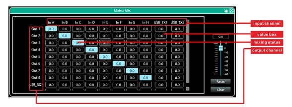
Input channel (on top side) corresponds to output channel. The box with a value is mixing key of channels. When the mixing key is cyan (double-click the value box to switch), the input channel and output channel signal realizes the mixing function.
