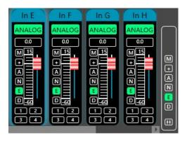
There are 3 kinds of input signal in device: ANALOG, Mic and testing signal. It will show a label for user.
