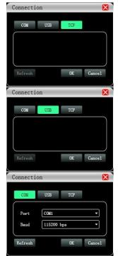
If connect device by using network cable, click Setting in Device List, choose TCP in Connection windows.
