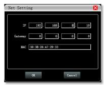
Set IP address of device refer to IP showed in the bottom of the software. Set the first three paragraphs same with the PC IP.
