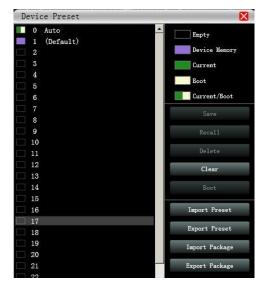
**Save**: select the saved gear, save all the parameter of the current automatic gear of the machine to the device preset (2~59 Preset bit).
