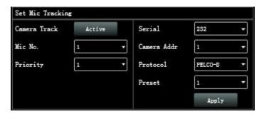
**Mic No.**: corresponds to the input channel of device. (parameter need to be set separately for each channel)
