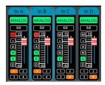
User can quickly set channels in groups for opening or closing mute, phase, noise gate, PEQ and delay function. AFC should be set independently, which can't be linked.
