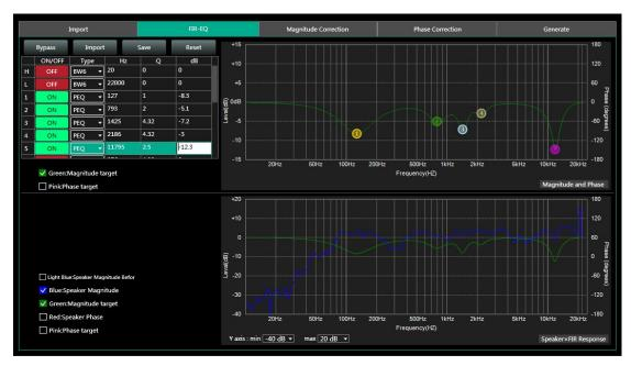
There are High pass filter and low pass filter for setting frequency divider, and 15 bands of PEQ \ LSLV \ HSLV to adjust magnitude. Try to set a linear magnitude of target speaker.
