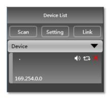
When using TCP control, there is a situation that only one point is displayed after scanning, but can not connect device. In this case, user need to change the IP address of the device to the same network segment as the PC computer.
